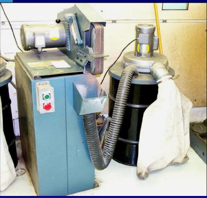
The belt sander generates particles which may be toxic. Use a sander with a vent attached and wear a mask before sanding work.
