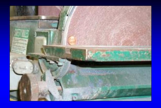
There is a pinch point where the sanding surface meets the table. The gap between them should be no wider than 1/16" (the width of a penny) to minimize this hazard.
