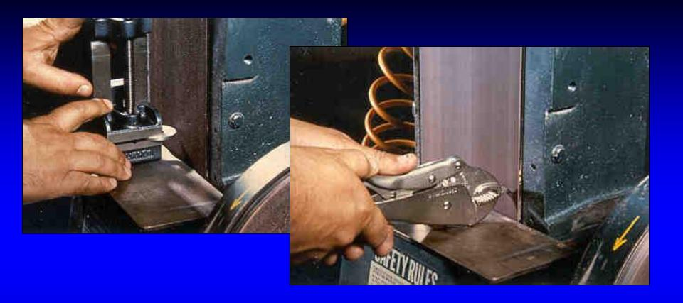
Avoid pressing the workpiece to the sanding belt with your fingers. Use a clamp or other tool to keep the point of contact at a safe distance.
