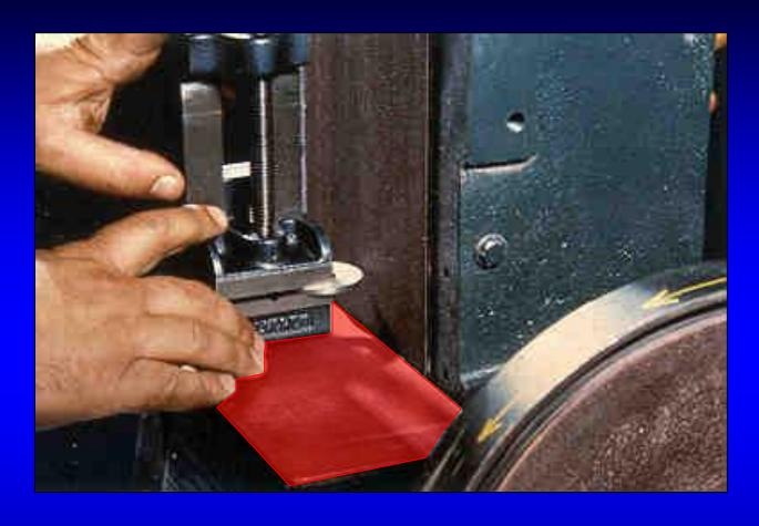
When smoothing edges and rounding corners of workpieces, the work should be supported on the table of the machine.
