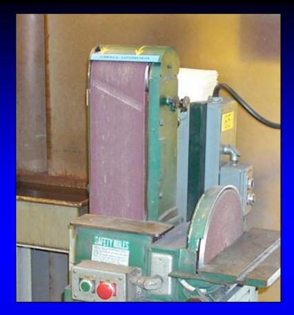
The belt sander is useful for removing burrs and rough edges from parts. It features an abrasive belt riding over two pulleys in a vertical motion. The sander pictured here also has an attached sanding wheel.
