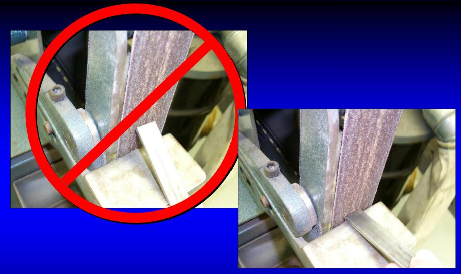
Always point the work down into the belt. This will prevent the belt from catching the workpiece and causing a possible injury.
